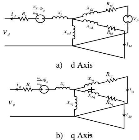
Fig. 1 Synchronous Machine Equivalent Circuits According to 2-2 Model of IEEE Std 1110
