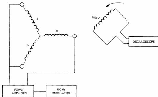
Fig. 2 Positioning rotor align with q-axis tests
