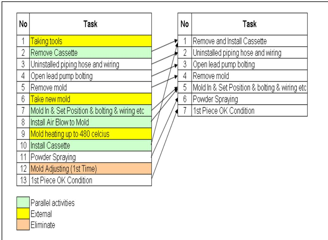
Figure 2: Tasks after SMED implementation in cast on strap
