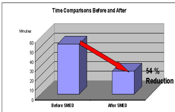
Figure 3: Time comparison before and after SMED implementation in cast on strap
