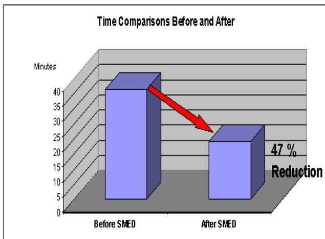
Figure 5: Time comparison before and after SMED implementation in heat seal
