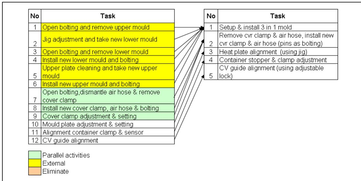
Figure 4: Tasks after SMED implementation in heat seal setup process
