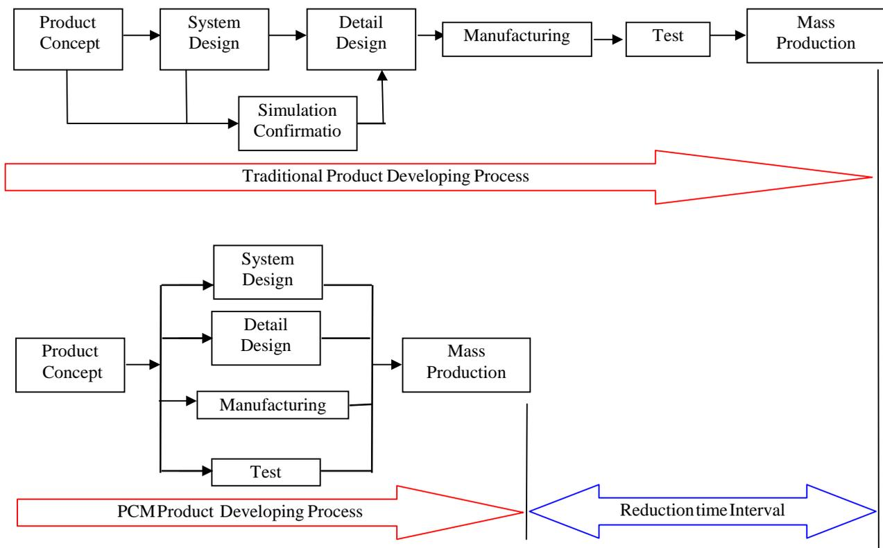
Fig. 2 The difference between traditional product developing process and PCM
