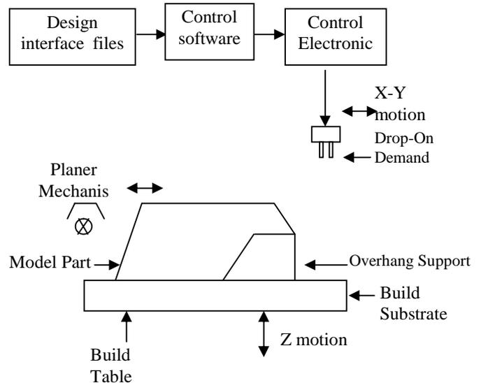
Fig. 5 The forming method of PCM prototype
