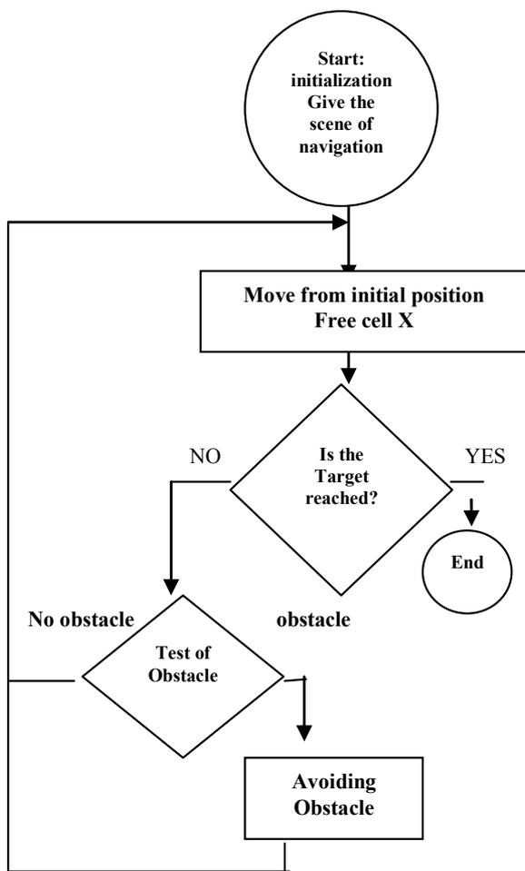
Fig.2 the general flowchart of the process of navigation of IAS
