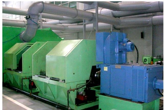
Fig. 4 brake performance dynamometer for high speed train
