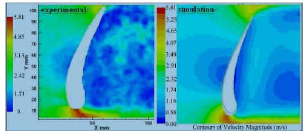
Figure 27 is the wind affect the vane produces contours velocity magnitude drawing (Angle of Attack  $\psi = 15^\circ$ )
