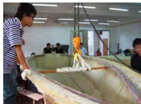
Figure 15 Finished product from the mold
