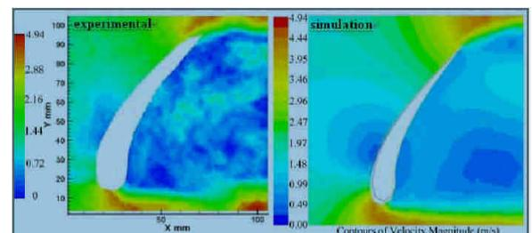
Figure 30 is the wind affect the vane produces contours velocity magnitude drawing (Angle of Attack  $\psi = 30^\circ$ )
