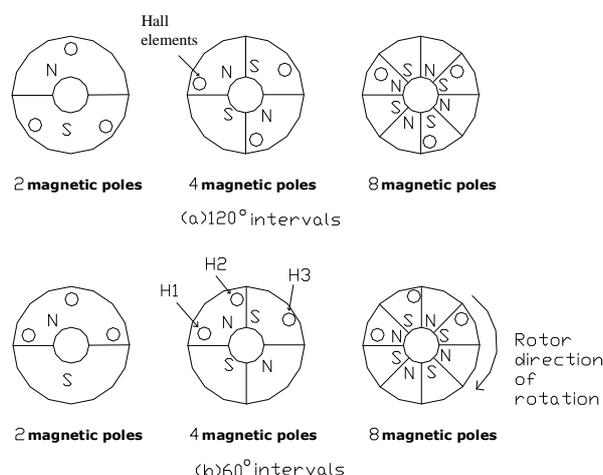
Figure 5 is Hall element adopts the rotor allocation with 120 or 60 degrees interval
