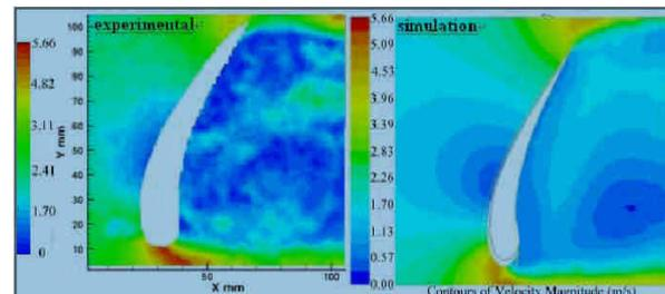
Figure 28 is the wind affect the vane produces contours velocity magnitude drawing (Angle of Attack  $\psi = 20^\circ$ )
