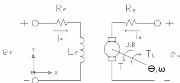
Figure 10. Field-controlled DC Motor System (including the load and damping) of the equivalent circuit [4]
