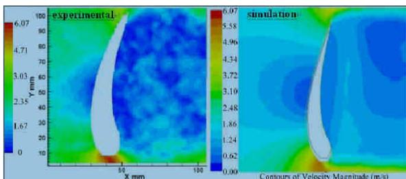
Figure 25 is the wind affect the vane produces contours velocity magnitude drawing (Angle of Attack  $\psi = 5^\circ$ )
