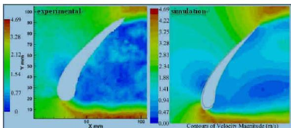
Figure 31 is the wind affect the vane produces contours velocity magnitude drawing (Angle of Attack  $\psi = 35^\circ$ )
