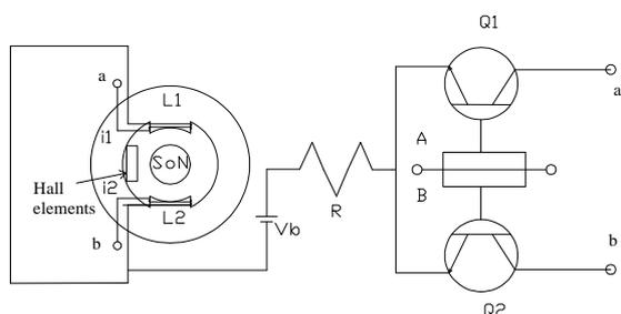
Figure 4 is BLDC Motor with Hall elements
