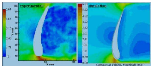
Figure 26 is the wind affect the vane produces contours velocity magnitude drawing (Angle of Attack  $\psi = 10^\circ$ )
