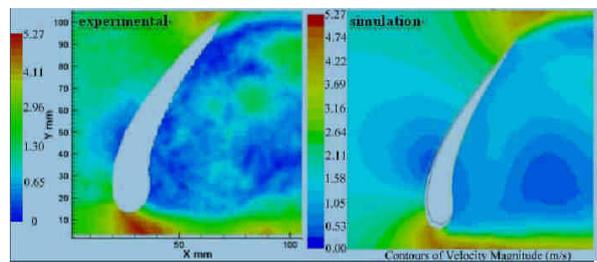
Figure 29 is the wind affect the vane produces contours velocity magnitude drawing (Angle of Attack  $\psi = 25^\circ$ )
