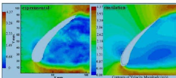
Figure 32 is the wind affect the vane produces contours velocity magnitude drawing (Angle of Attack  $\psi = 40^\circ$ )
