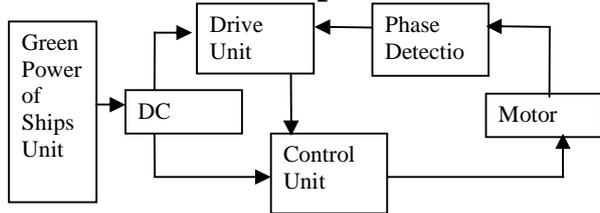
Figure 11. Diagram of BLDC Motor application in Green Power Ship.
