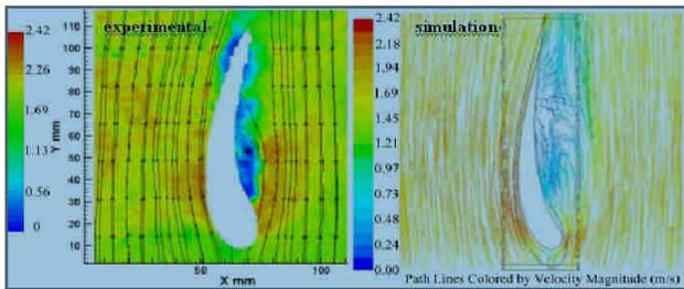
Figure 23 is the vane tangent directions to path lines colored by velocity magnitude drawing.
