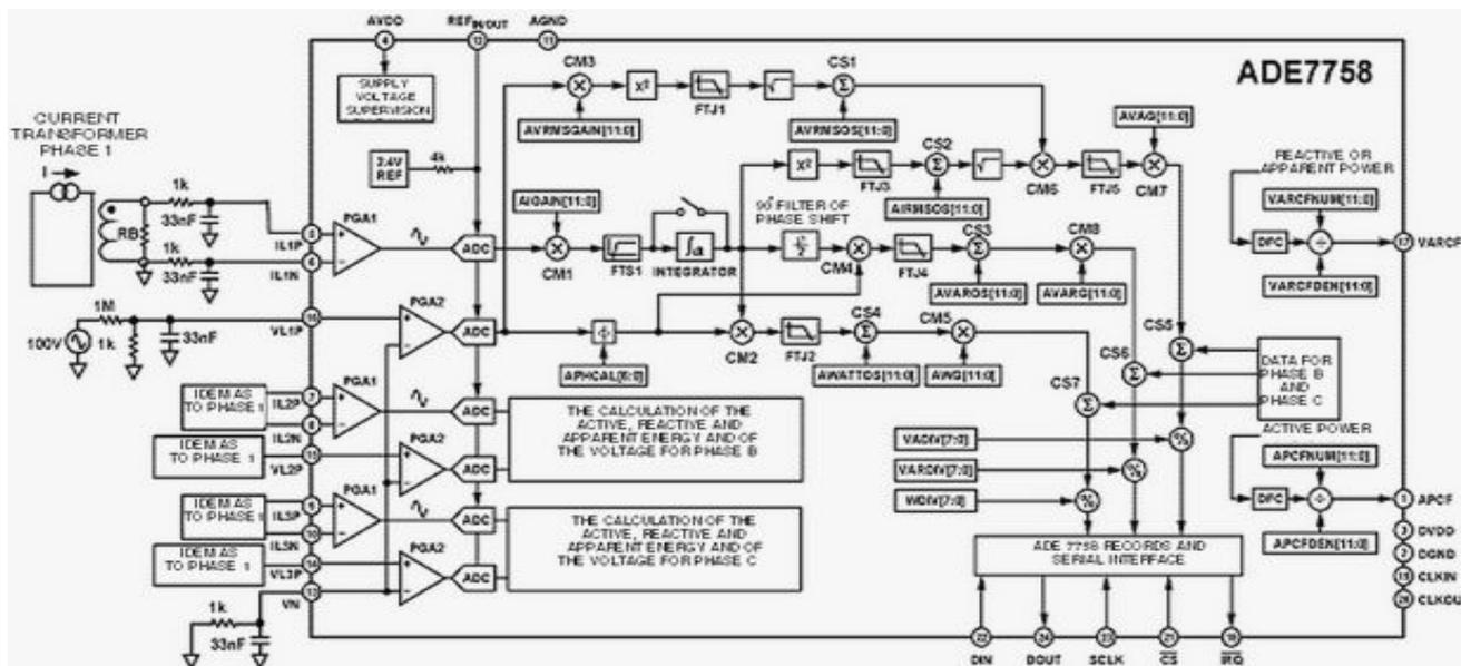
Fig. 5: Block diagram of the module to adapt and processing analog magnitudes.
