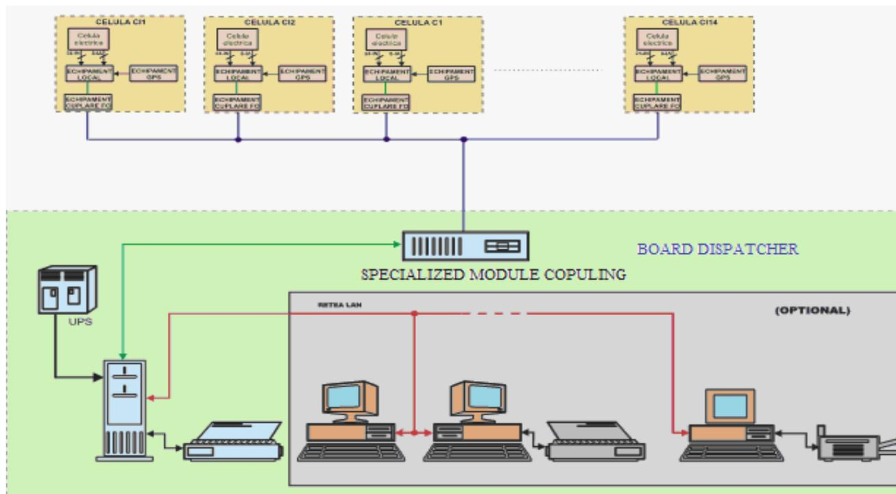
Fig. 2: Block diagram: recording system energy quantities of electric power stations.
