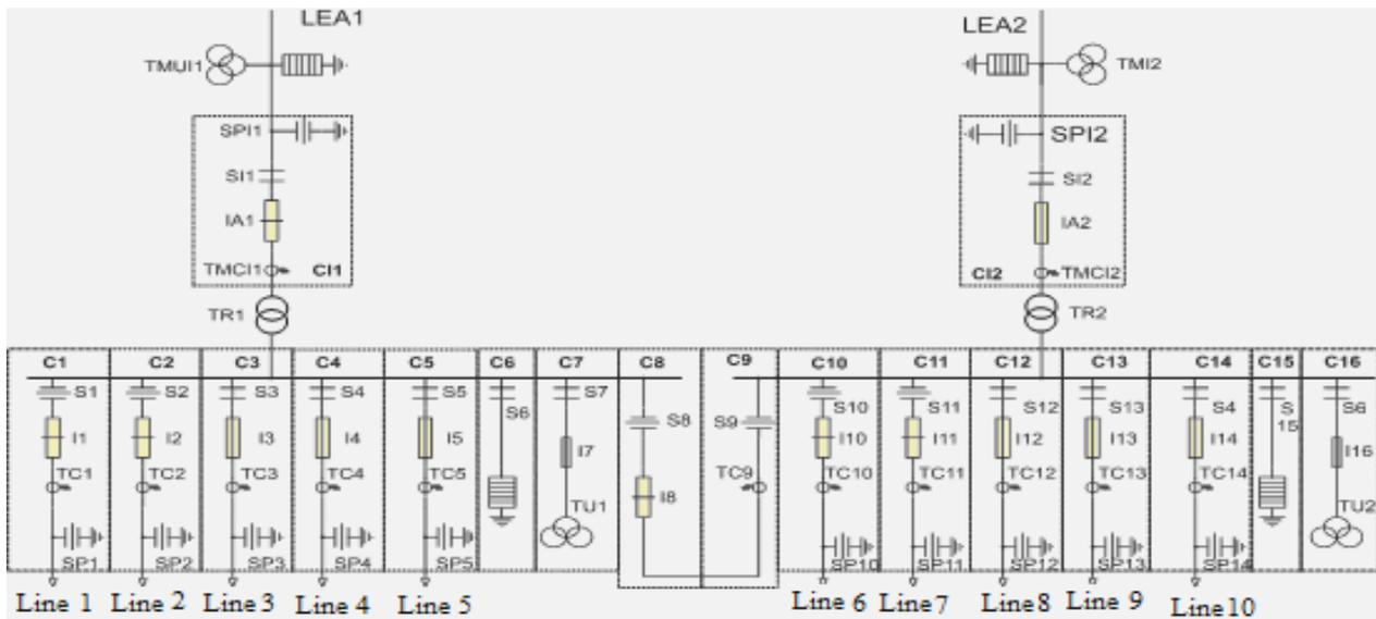
Fig 1: Monofiber schedule for power transformer station.
