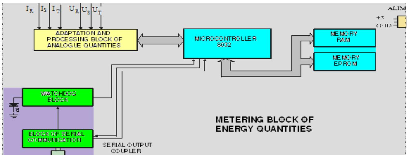
Fig. 4: Block sizes measuring energy.
