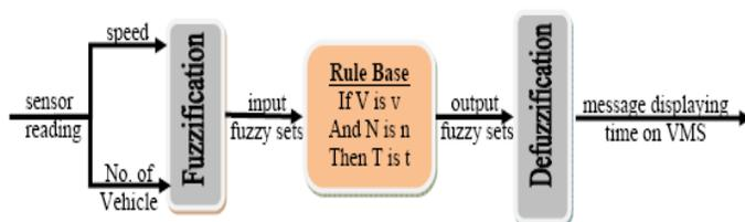
Fig. 4 Fuzzy Logic Controller, block diagram
