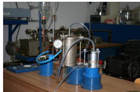
Fig. 7 Constant head permeameter without suction
