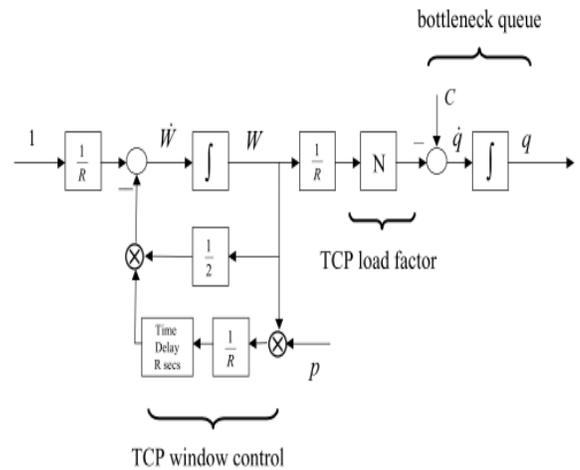
Fig.3 Block-Diagram of TCP connection
