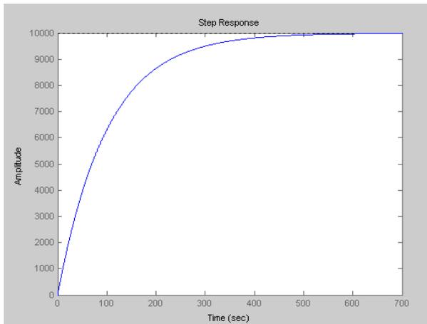
Fig 11. Step response of the closed loop obtained with mixed  $H_\infty$  controller
