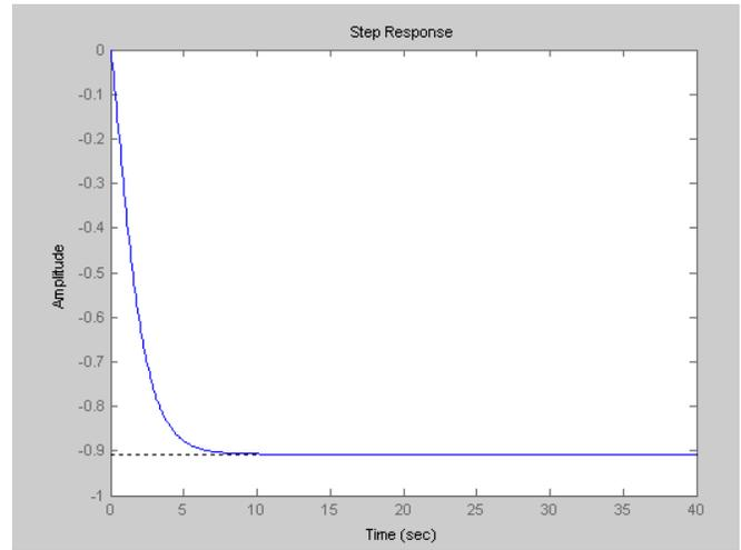
Fig 8. Step response of the closed loop obtained with H2 controller
