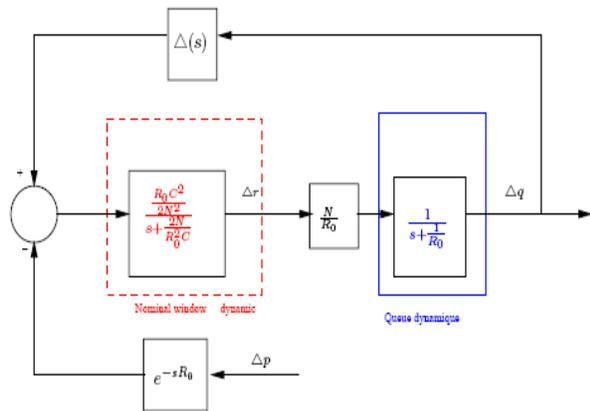
Fig.6 Block diagram representation of model uncertainties of TCP/IP flow under uncertainties
