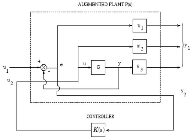
Fig 10. Closed loop transfer function for mixed sensitivity
