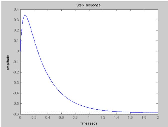
Fig 9. Step response of the closed loop obtained with  $H_\infty$  controller
