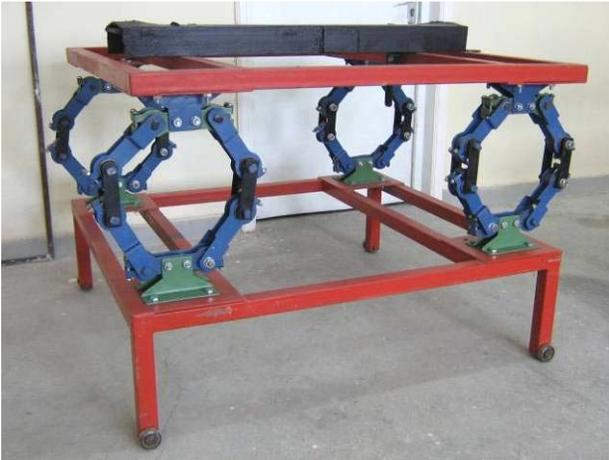
Fig. 10. The special elastic systems with polygonal configuration - singular montages
