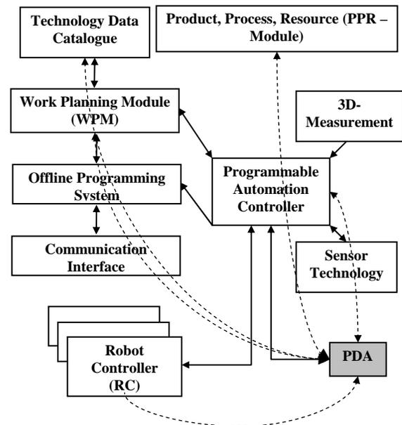
**Fig. 7 Robot control system with PDA**
