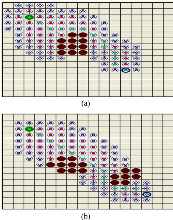
Figure 5. The result of A\* search algorithm for obstacles in different situations
