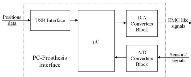
Fig.7 PC-Prosthesis interface block diagram
