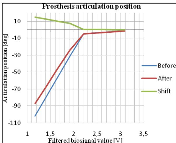
Fig. 11 Auto calibration effect over prosthesis articulation position
