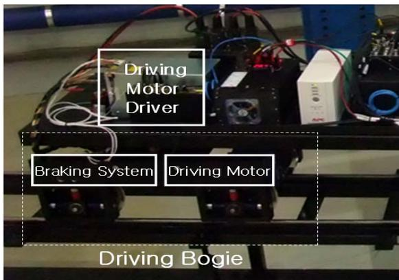
Fig.7 a driving bogie module
