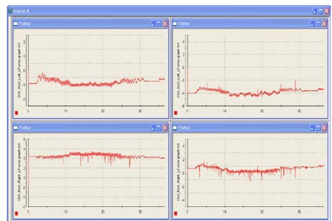
Fig. 17 the experimental results: the lateral force of the wheel using the measuring system in case of applying the displacement control strategy
