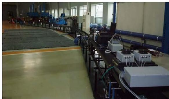
Fig.4 research test-bed: the 1/5 scale active steering vehicle and the curved track
