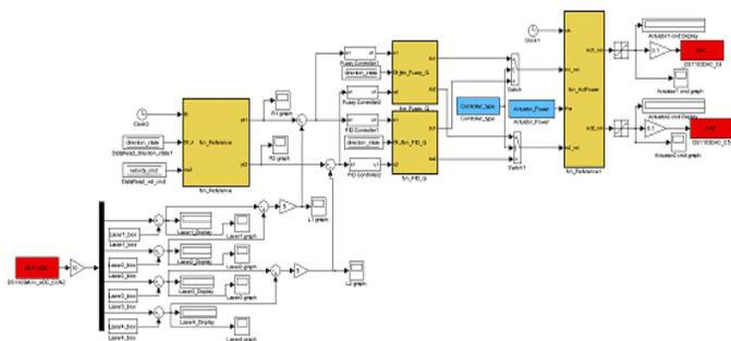
Fig.3 realization of the active steering control module with MATLAB/SIMULINK
