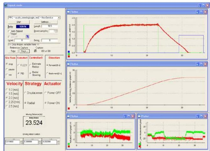
Fig. 16 the experimental results: the moving distance of the driving axle and braking axle
