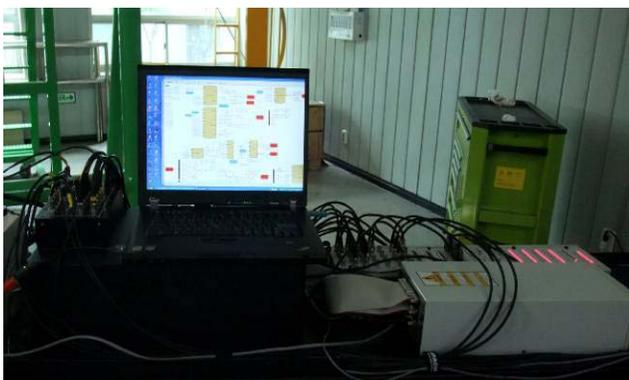
Fig.8 an active steering controller (DS1103 PPC Controller Board and desktop PC)
