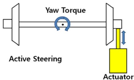
Fig. 2 active steering control strategy: longitudinal actuator method
