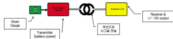
Fig.12 the signals flow and bridge circuits for the measuring the wheel load and the lateral force
