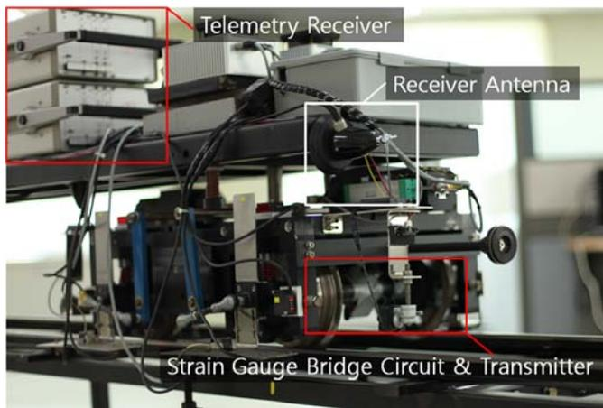
Fig. 14 lateral force measuring system
