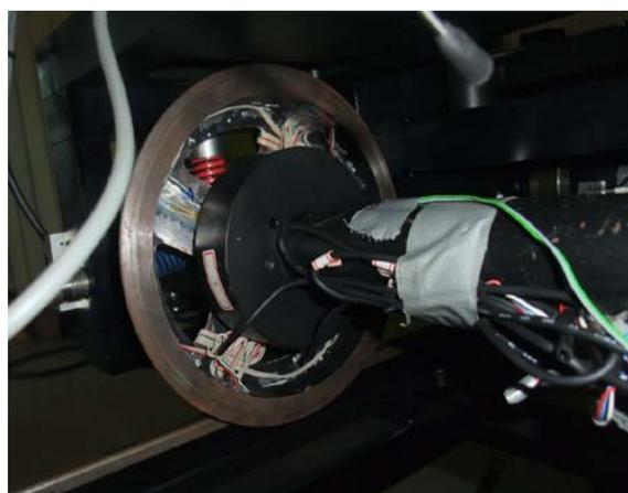
Fig. 15 a prototype of the lateral force measuring system which contains bridge circuits, signals transmitter, antenna, and battery
