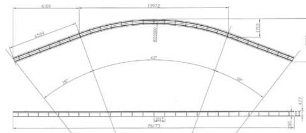
Fig.5 drawings of the curved track of test-bed for running test for active steering control system
