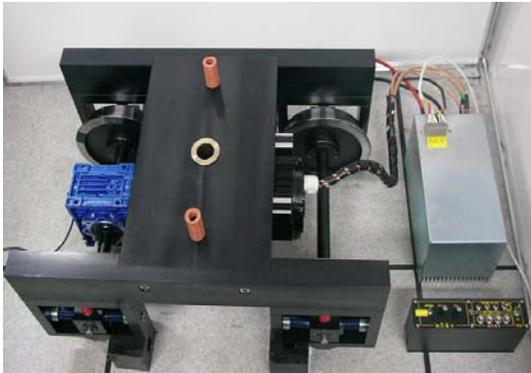
Fig.6 a driving motor and a motor driver
