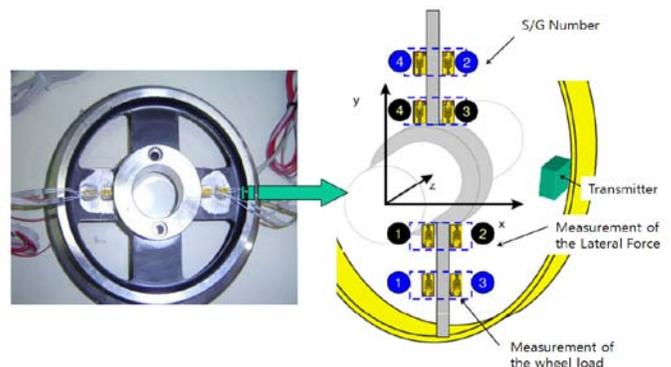
Fig. 13 lateral force measuring system and its prototype
