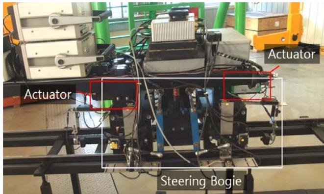
Fig.10 an active steering bogie module
