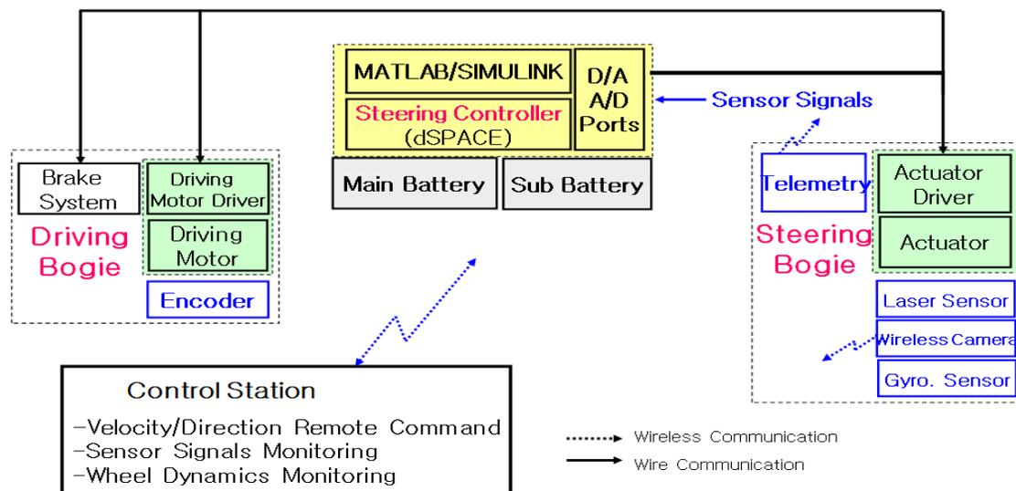
Fig. 1 block diagram of the proposed active steering control systems
