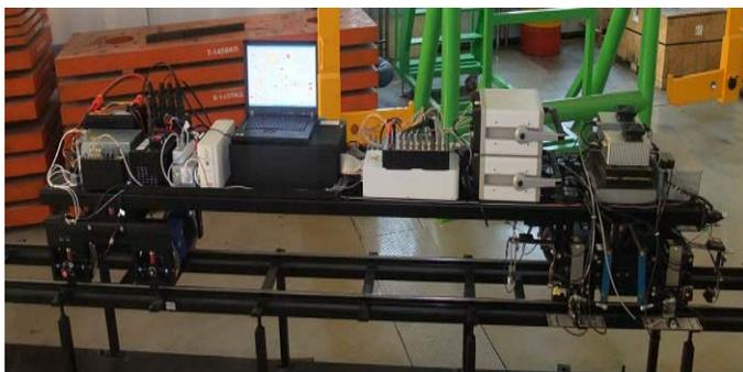
Fig. 11 the scaled vehicle with various sensor systems
