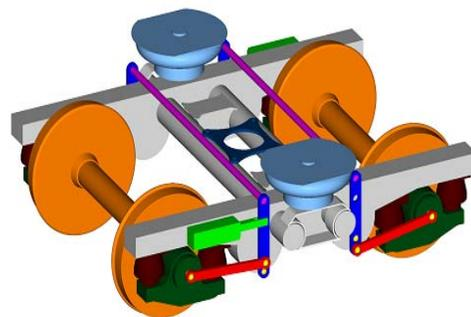
Fig.9 schematic views of the active steering bogie module
