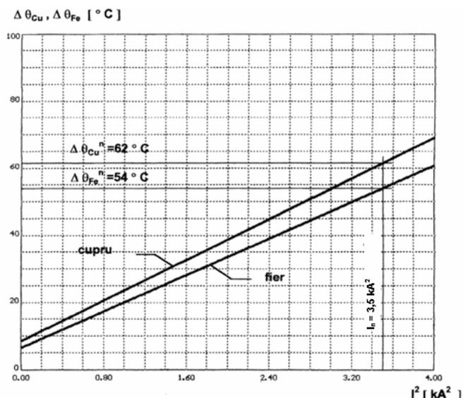
Fig. 2: Characteristic thermal stator winding and stator core of hydro generator.
