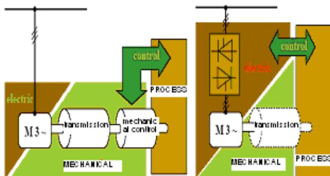
Fig.3. Reducing power losses in electrical drives by the shift from mechanical control (a) to power control (b).
