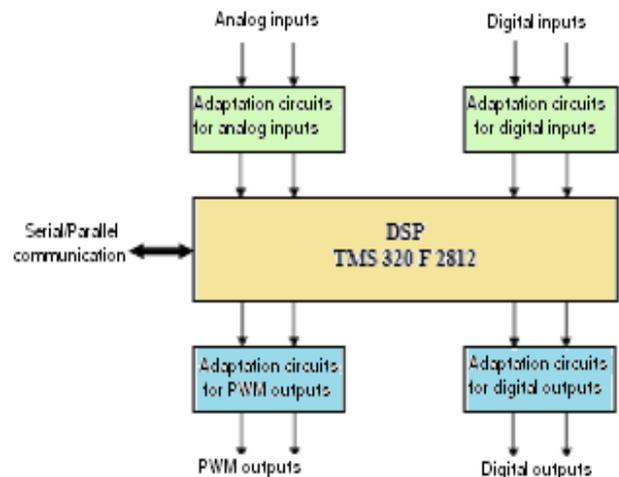
Fig. 8: Block diagram of the development platform TMS 320 F 2812\* .
