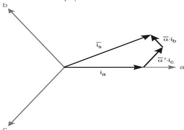
Fig. 4: The diagram of spatial phaser for the stator current.
