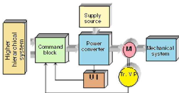
Fig. 2: The block diagram of an electric drive system.
