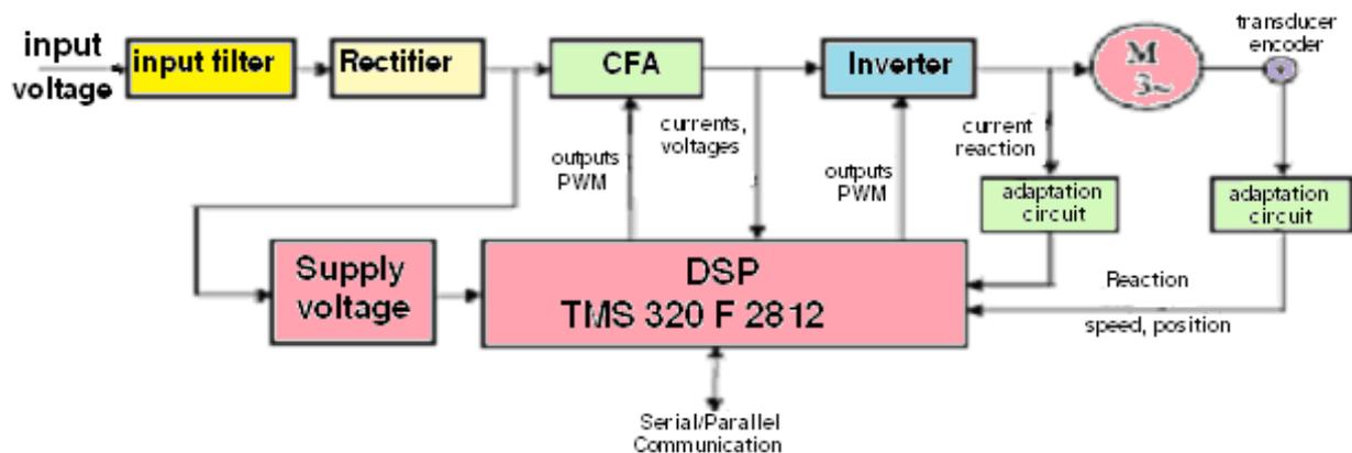
Fig. 5: The block diagram of an electric drive system with DSP and AC engine.
