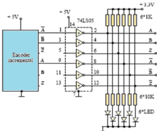
Fig. 7: The proposed circuit for adaptation of incremental encoder signals to DSP.
