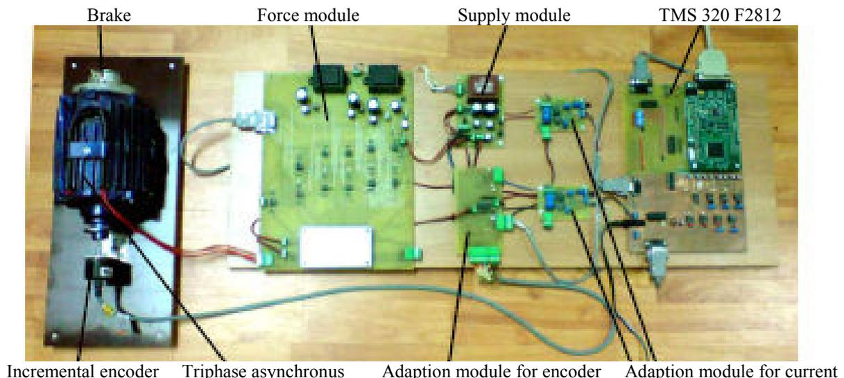
Fig. 10: Realization of electric drive system with DSP and AC engine [3].
