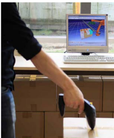
Fig. 9 positioning of the parcels by a “6 DOF-tracking device”
