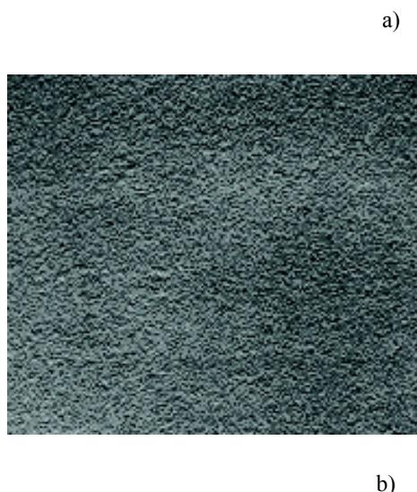
Fig. 2. Electron microscope images of the surface of  $Pb_{1-x}Mn_xTe$  ( $x=0.02$ ) epitaxial films; a) without additional compensating Te vapors source, b) with additional compensating Te vapors source.
