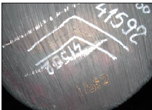
Figure 4. Central internal fissures
