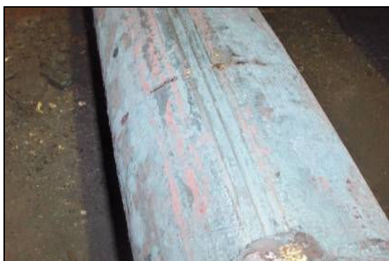
Figure 17. Dent of roller
