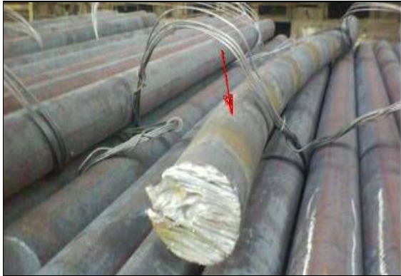
Figure 16. Bars showing a curvature defect
