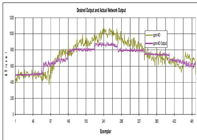
Figure 8. Desired output and actual network output about NO
