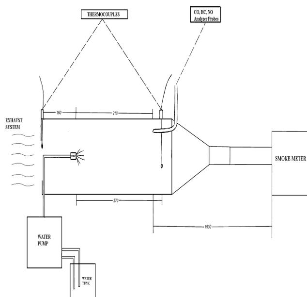
Figure 2. Layout of exhaust with the injector (beck) internal.
