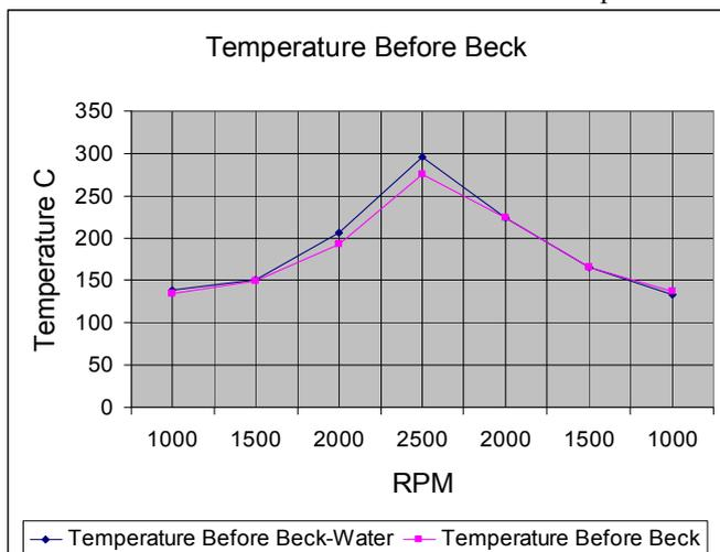
Figure 16. The average mean value of gas emissions temperature before injector (beck) with and without spraying of water, in relation to rounds in rpm.
