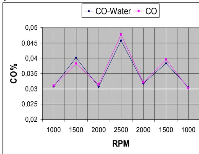
Figure 19. The average mean value of CO % emissions with and without spraying of water, in relation to rounds in rpm.
