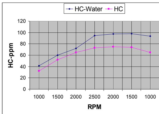
Figure 20. The average mean value of HC-ppm emissions with and without spraying of water, in relation to rounds in rpm.
