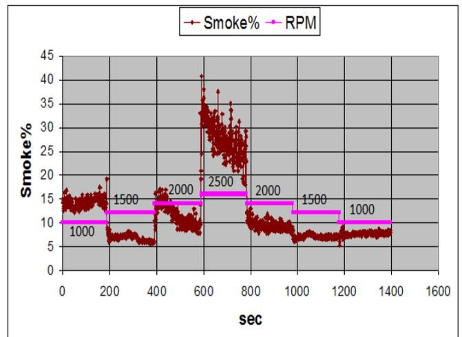
Figure 8. The percentage (%) of smoke emissions, without spraying of water, in relation to time in seconds and rounds in rpm.
