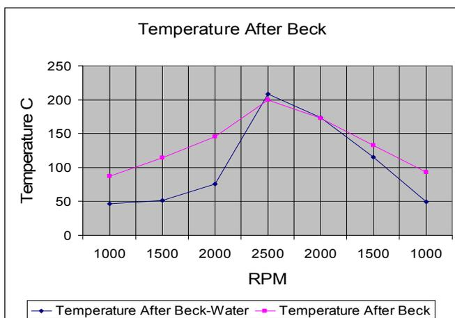
Figure 17. The average mean value of gas emissions temperature after injector (beck) with and without spraying of water, in relation to rounds in rpm.
