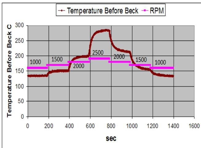
Figure 4. Gas emissions temperature before beck, without spraying of water, in relation to time in seconds and rounds in rpm.
