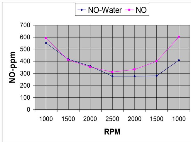
Figure 21. The average mean value of NO-ppm emissions with and without spraying of water, in relation to rounds in rpm.
