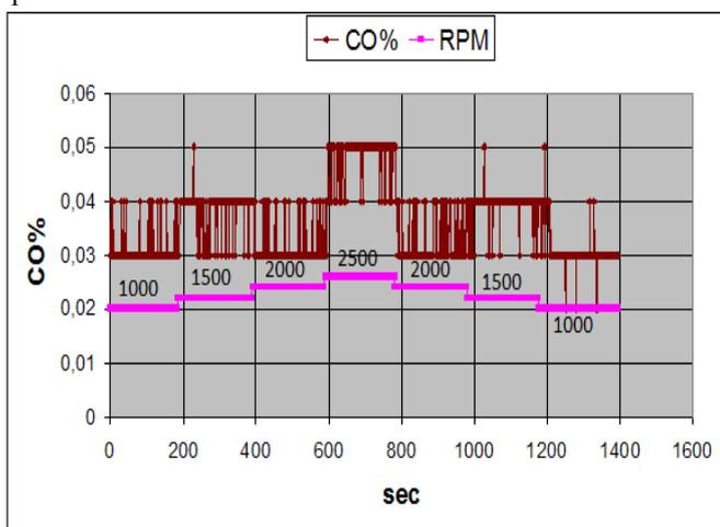
Figure 10. The percentage (%) of CO emissions, without spraying of water, in relation to time in seconds and rounds in rpm.
