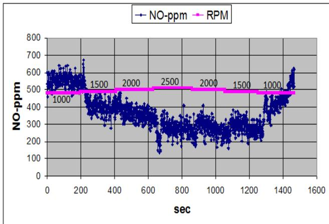
Figure 15. The NO-ppm of gas emissions with spraying of water in relation to time in seconds and rounds in rpm.
