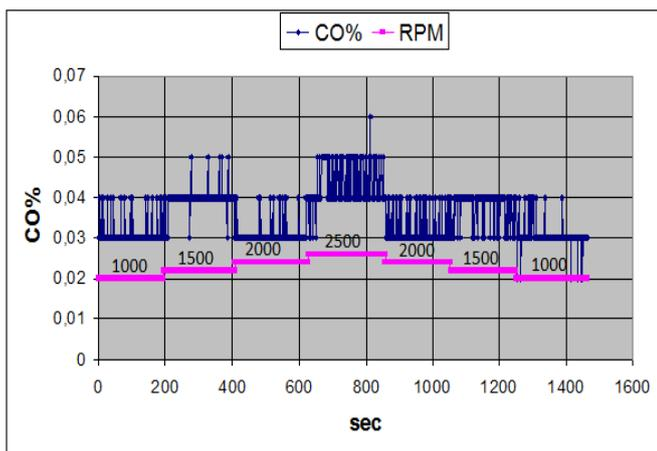
Figure 11. The percentage (%) of CO emissions, after spraying of water, in relation to time in seconds and rounds in rpm.
