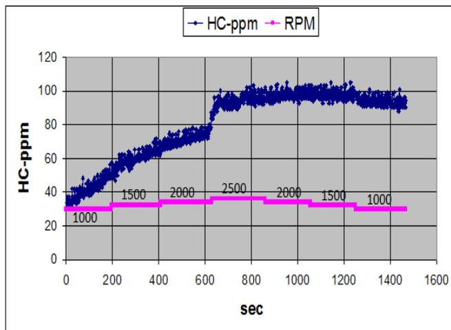
Figure 13. The HC-ppm of gas emissions with spraying of water in relation to time in seconds and rounds in rpm.
