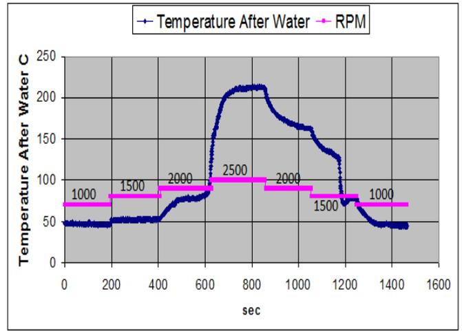
Figure 7. Gas emissions temperature after beck, after spraying of water, in relation to time in seconds and rounds in rpm.
