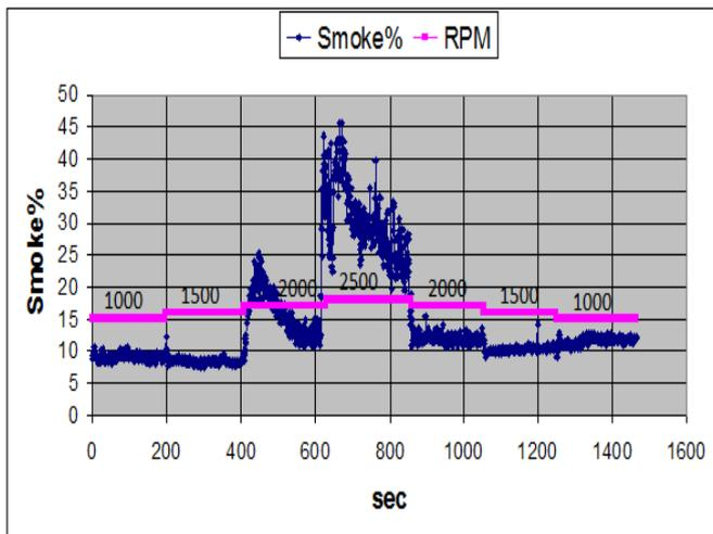
Figure 9. The percentage (%) of smoke emissions, with spraying of water, in relation to time in seconds and rounds in rpm.
