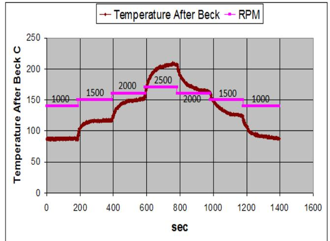
Figure 6. Gas emissions temperature after beck, without spraying of water, in relation to time in seconds and rounds in rpm.
