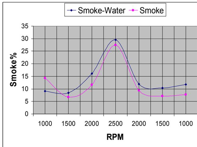
Figure 18. The average mean value of smoke % emissions with and without spraying of water, in relation to rounds in rpm.
