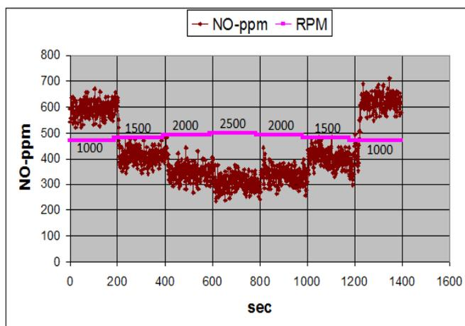
Figure 14. The NO-ppm of gas emissions without spraying of water in relation to time in seconds and rounds in rpm.
