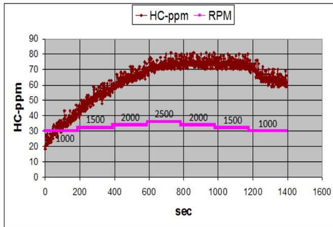
Figure 12. The HC-ppm of gas emissions without spraying of water in relation to time in seconds and rounds in rpm.
