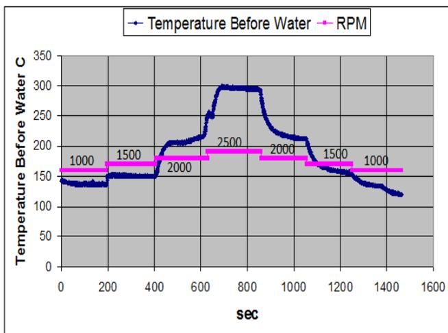
Figure 5. Gas emissions temperature before beck, with spraying of water, in relation to time in seconds and rounds in rpm.
