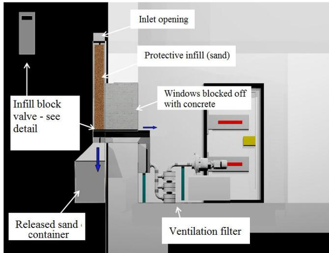
Legend: the direction of material movement (sand) and a retractable board securing the filling
