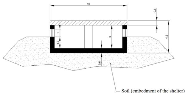
Figure 5: Side view of the IS without modifications
