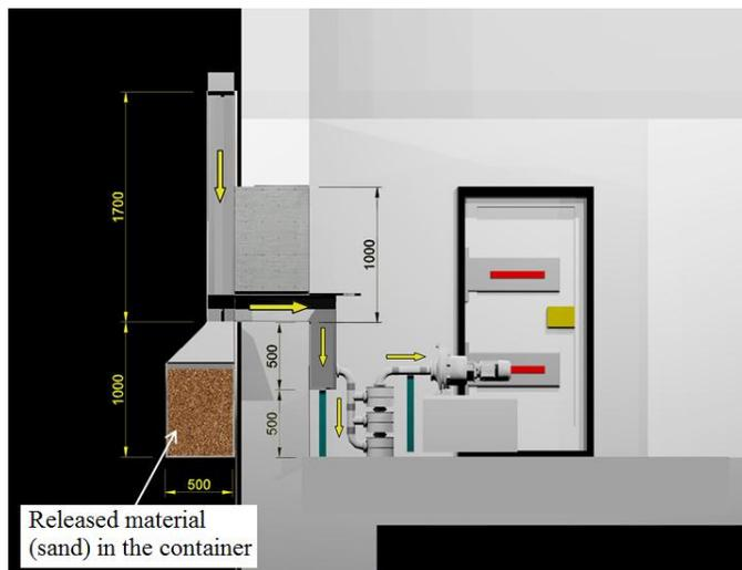
Legend: a direction of air movement into the interior of the shelter
