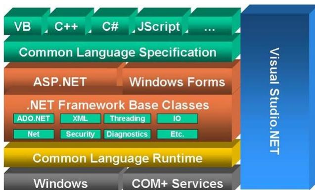
Fig. 3 - Architecture .NET Framework, Source: [12]
