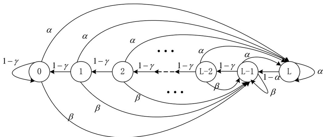
Fig. 2 The proposed L-state bursty channel model
