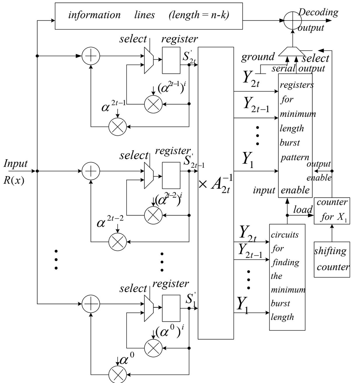
Fig. 6 VLSI hardware decoder structure for the proposed burst-error-correcting algorithm
